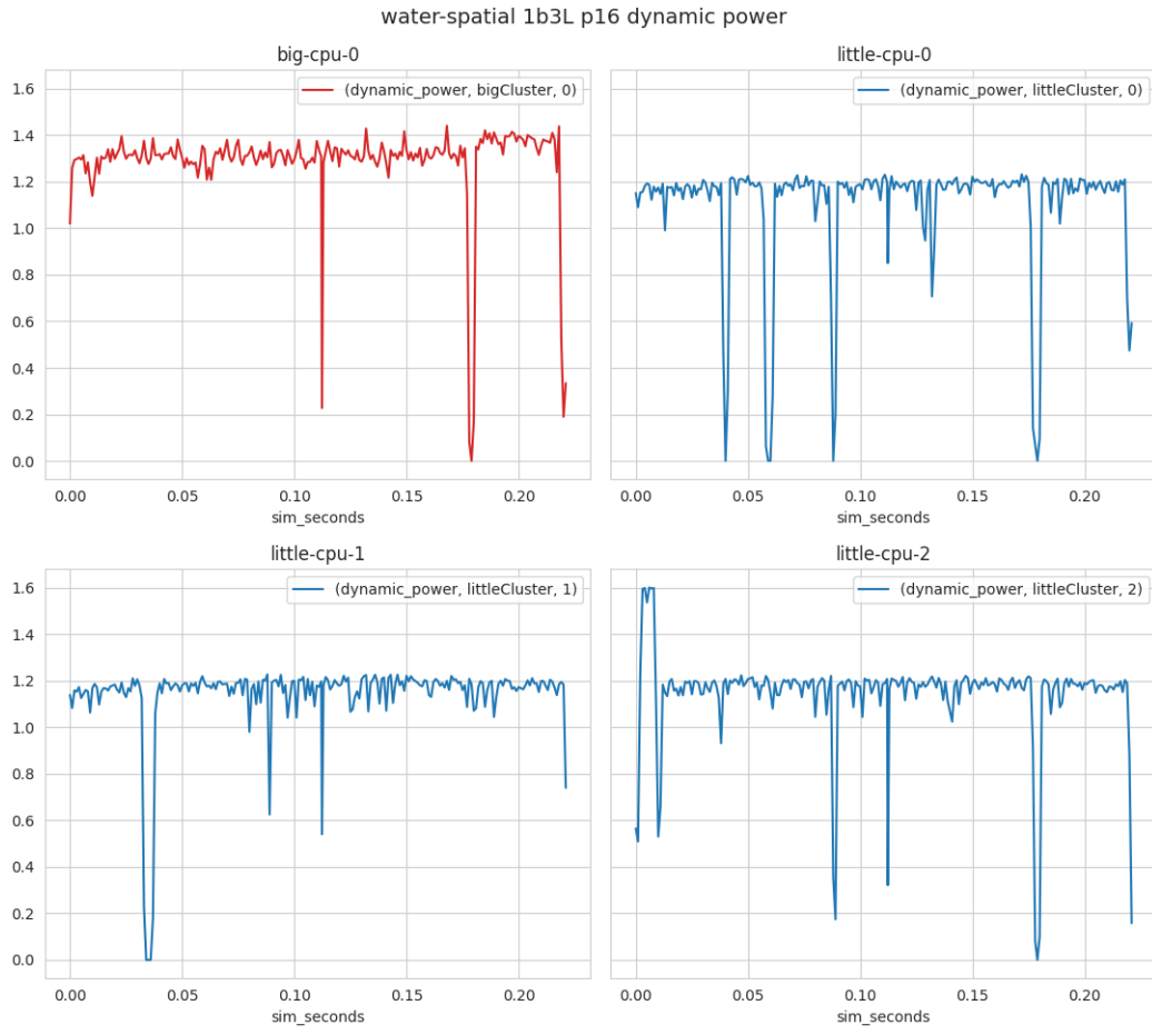
Figure B.11: Dynamic power for 16-threaded water-spatial on 1 big 3 LITTLE cores (completed)
